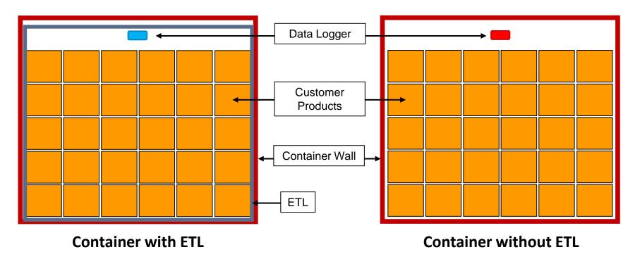
Containers with and without ETL were each loaded with bags filled with food emulsifier and the temperature data loggers were placed at the top area inside the containers. Both containers were sent side by side to the same destination.
